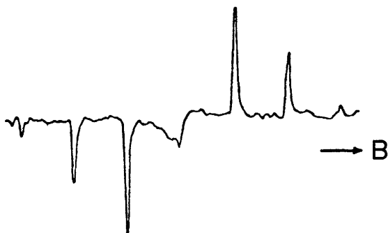
Figure 1 Multiplet ST_0 radical pair polarization in the (\text{CH}_3)_2\text{COH} radical formed on the flash-photolysis of benzophenone in propan-2-ol solution (A. D. Trifunac et al. 12 ). The field increases from left to right and the unpolarized central line is distorted by overlap of an emissive signal from the benzophenone ketyl radical. This unusual e.s.r. spectrum was obtained as a field profile (see Figure 7) without field-modulation which normally yields the derivatives of the lines shown. Often in multiplet patterns comparatively small polarizations result in the intensity distribution appearing unsymmetric about the centre, due to significant contributions from equilibrated radicals present
